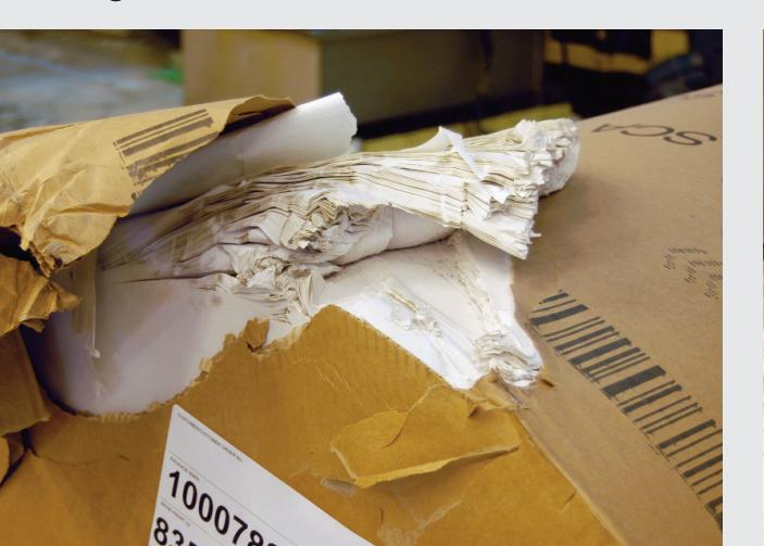
The roll has been standing or pushed onto stones, or other foreign material, during transit; or lowered to ground in tilted position.
