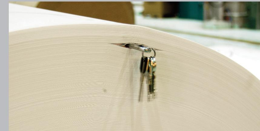
Variations in sheet thickness across the web (or both) creates a "long edge" which cannot be tensioned in the winder. An area of paper across the width of the web appears slack or baggy and can result in creasing; loss of register, and web wander (especially over air toner bars).
