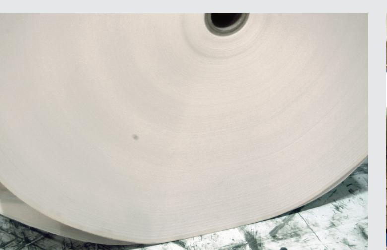
Caused by hard impact during transit; prolonged horizontal storage; excessive clamp truck pressure.
