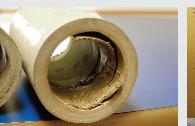
Delaminated core can be caused by poor pressure on the expanding chucks or the roll have been put in or out several times in the press or poor/wrong core quality.
