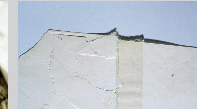
Poor mill joint: The splice tape is incorrectly positioned and sticks to the paper underneath. Protruding mill joint: Webs are not line-up with each other and the paper protrudes at the edge of the roll. Stuck mill joint: The splice tape is not covered by the paper and sticks to the paper layer causing a break.
