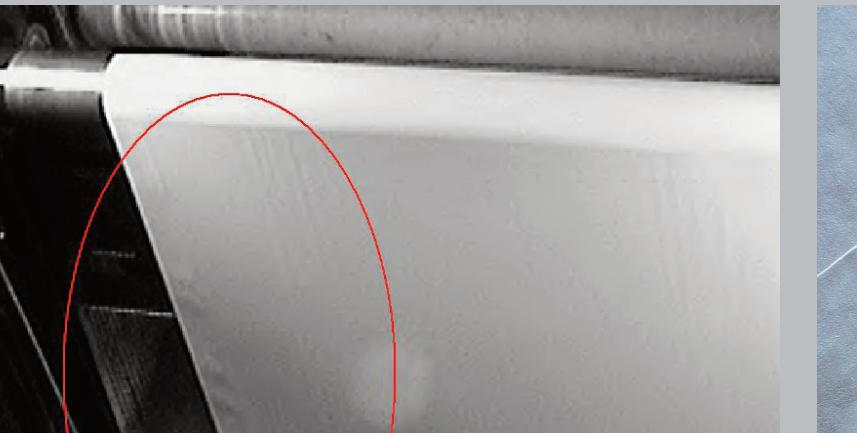
Poor moisture or caliper profile across the web (or both) creates a "long edge" which cannot be tensioned in the winder. An area of paper across the width of the web appears slack or baggy and can result in creasing; loss of register, and web wander (especially over air toner bars).
