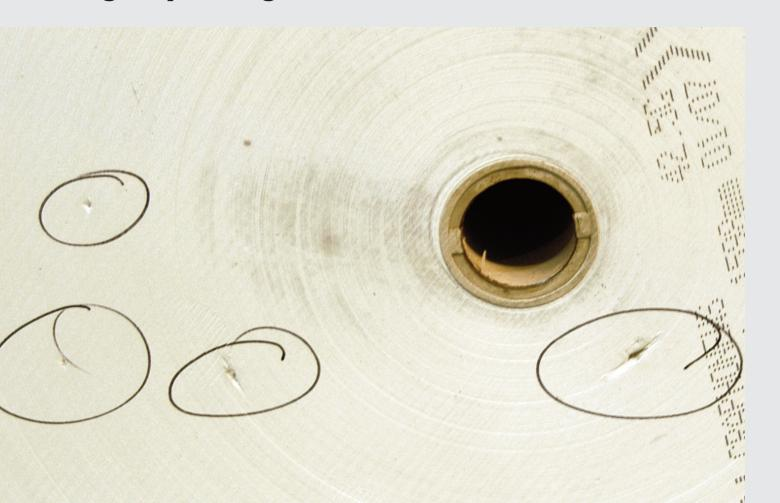
Indent to the edge of the roll. Usually fixed by grinding off damage.
