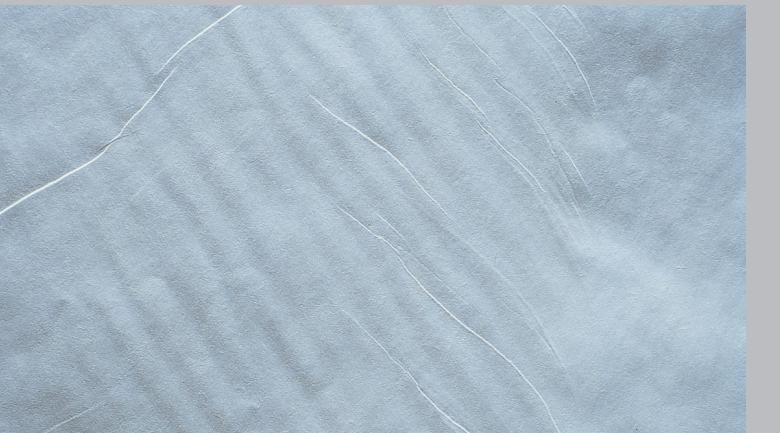
These occur when areas with different caliper cause the web to stretch under high tension during winding and/or unwinding. They are bands of relative variation which extend around the roll, parallel to the machine direction, and possibly all the way through the roll. Between these bands are diagonal markings that resemble a rope or have a tyre-like pattern.
