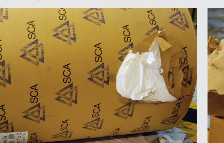
Perforation of body wrapping and paper by poor handling (scuffing, impact against a sharp object, incorrect clamp truck procedures).
